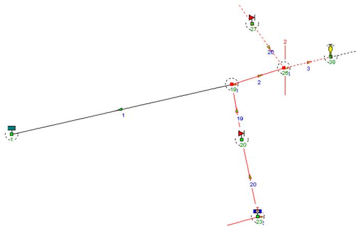
Detail of the calculation model, with valve, backflow prevention valve, aeration and deaeration
